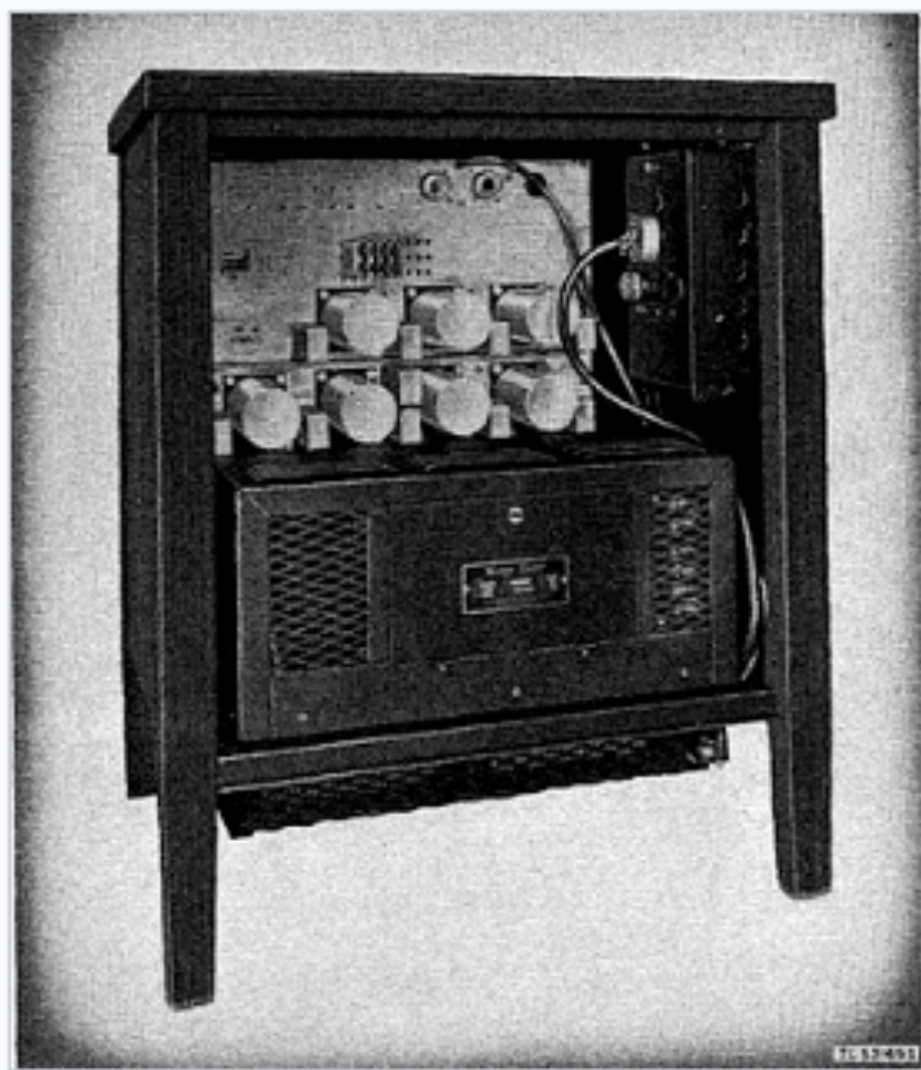
Bell 131B2 mixer, used to XOR teleprinter signals with one time tapes, was the first device from which classified plain text was extracted using radiated signals.
